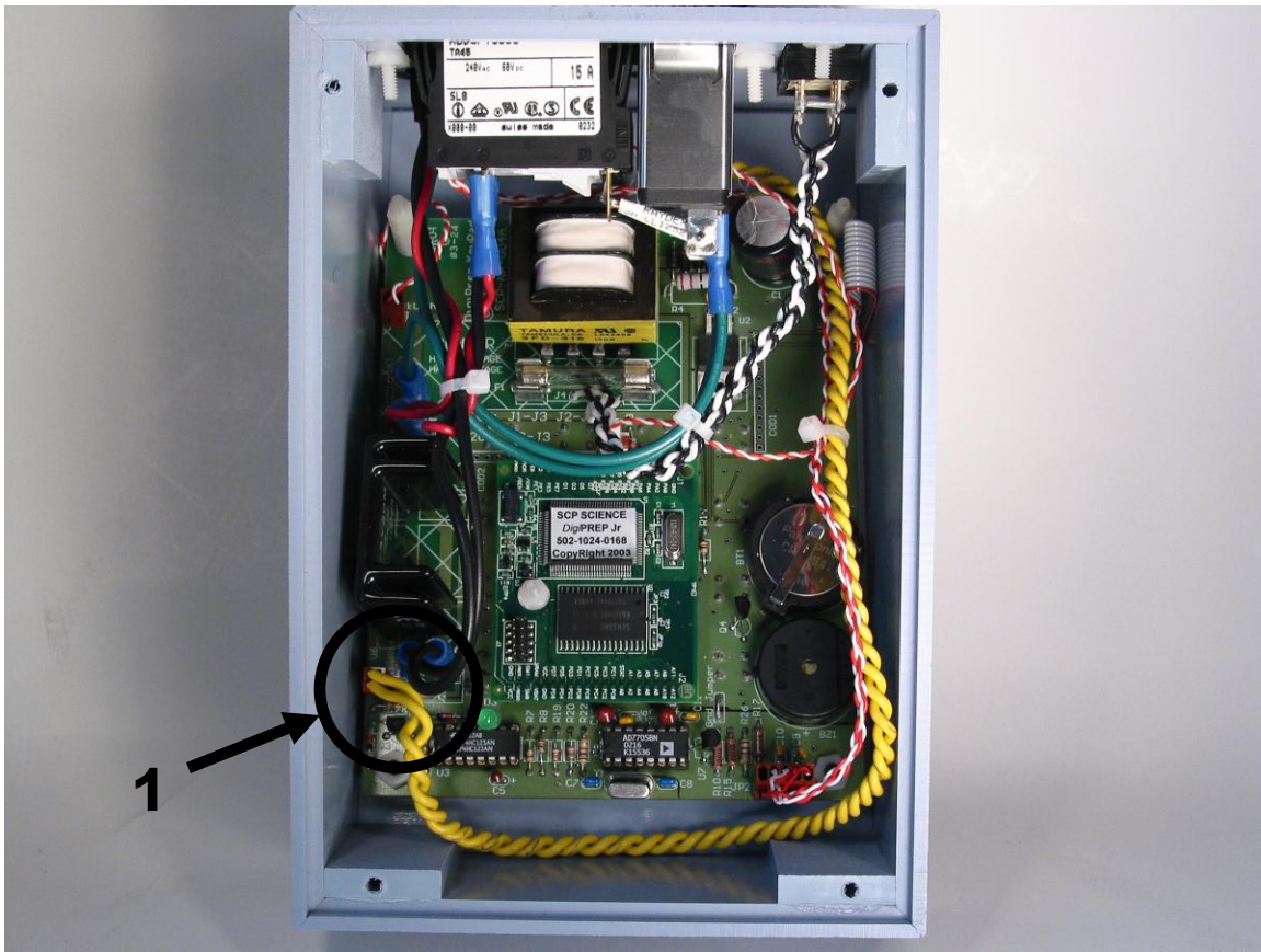
Figure 16: DigiSET connector location
