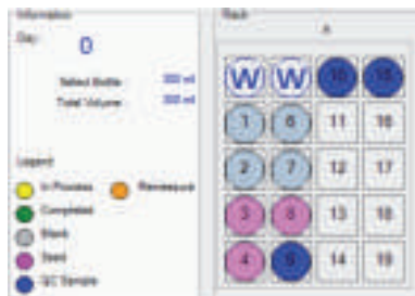
Figure 32. Incorrect pairing of QC/sample in the process list.
