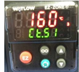
Figure 3. High temperature setting for timed heating cycle
