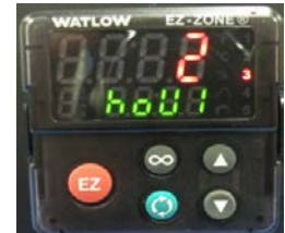
Figure 4. Digital hour readout for timed heating cycle
