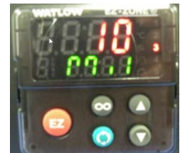
Figure 5. Digital minute readout for timed heating cycle
