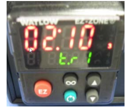
Figure 6. Digital readout for "time remaining" for timed heating cycle
