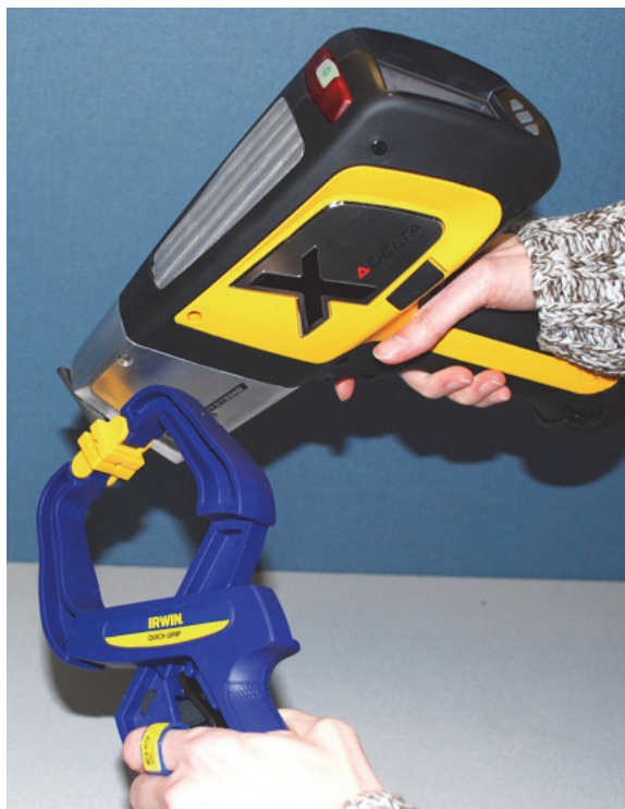
Figure 2-5 Sample held by a clamp
