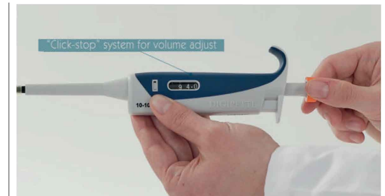
“Clik-stop” mechanism of volumen selection
