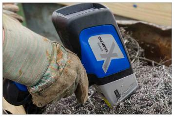
When reliable material analysis is required, the DELTA Element provides fast and accurate Positive Material Identification (PMI). To confirm that installed pipes and fittings are the specified material, the DELTA enables testing anytime, anywhere for fast, accurate results.
