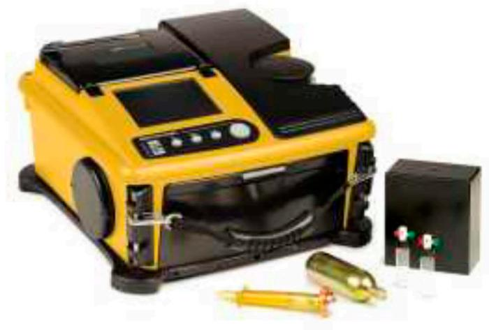
*The TRIDION-9 GC-TMS was engineered for ease of use, speed and portability.*
