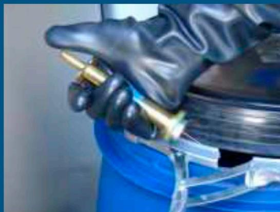
Not only is SPME a flexible tool to use for sampling, but Torion also designed the CUSTODION Syringe to house the SPME fiber with safety and simplicity in mind. With a click of the plunger the SPME fiber is exposed and retracted, as easy as clicking a ball point pen. Users wearing thick protective gloves can still easily operate the CUSTODION Syringe. The CUSTODION Syringe is universal and can be used with any laboratory GC.
