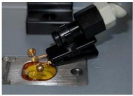
In addition, analyzing dental gold by using conventional gold-purchase acids is difficult; the acid method which works for jewelry might not necessarily work for dental alloys, as they contain non-traditional alloying elements. The optimal analysis method for assaying dental alloys is X-Ray Fluoresence (XRF), a fast, precise, and nondestructive analytical technique.
