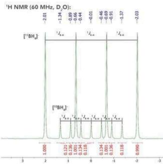
Figure 1. <sup>1</sup>H NMR Spectrum of NaBH<sub>4</sub> in D<sub>2</sub>O.
