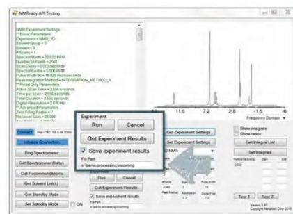
Step 2: Connect NMReady Automation tool to spectrometer & configure it to write to MNova listener folder
