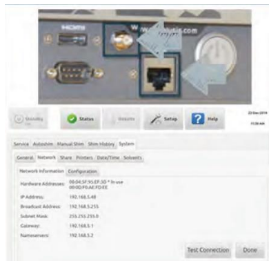
Step 1: Network the NMReady spectrometer with Ethernet or Wi-Fi connectivity
