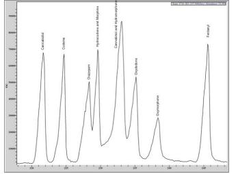
*Figure 2.* Chromatogram showing the co-elution of hydrocodone/morphine and cannabinol/hydromorphone.
