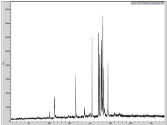
Figure 4. Chromatogram of all 16 drugs when dipping the CWF into a drug mixture (60  $\mu g/mL$  of each drug).
