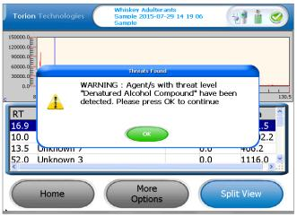
*Figure 2.* An example of an 'Alert' when a target compound in denatured alcohol is detected.
