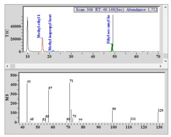
*Figure 1.* Chromatogram and mass spectrum, with identification of marker components in a Euro spike of a blended Scotch Whisky
