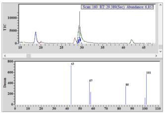
*Figure 4.* Chromatogram from single malt Scotch whiskey showing detection and identification of methyl isobutyl ketone (MIBK) co-eluting with a flavor/aroma compound.
