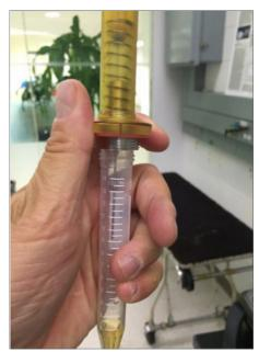
*Figure 3.* Sampling with the CUSTODION. The SPME fibre is housed in a durable syringe that is operated like a ball point pen.
