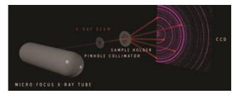
These instruments use patented technology developed for the NASA Mars Rover project and off er some unique features compared to conventional XRD that makes them well suited for the academic environment.
